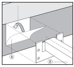
■ Position and attach the spring clips
